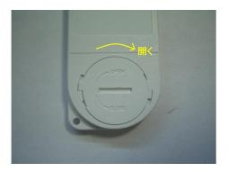
Hold the back of the case downwards, magazines etc. If you hit lightly on objects of moderate hardness, the back lid and batteries will come off.
